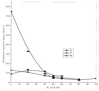
**Figure 13** Effect of the blend ratio and different crosslinking systems on the relative volume loss of the SBR/EVA blends.
