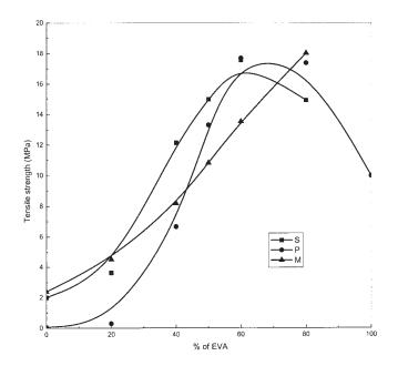
Figure 8 Effect of the blend ratio and different crosslinking systems on the tensile strength of the SBR/EVA blends.
