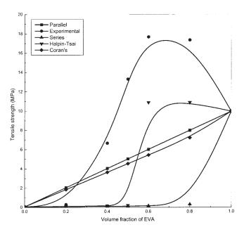
**Figure 15** Applicability of various models on the tensile strength of the DCP-cured SBR/EVA blends.
