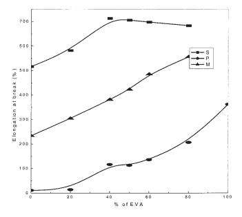
**Figure 10** Effect of the blend ratio and different crosslinking systems on the elongation at break of the SBR/EVA blends.
