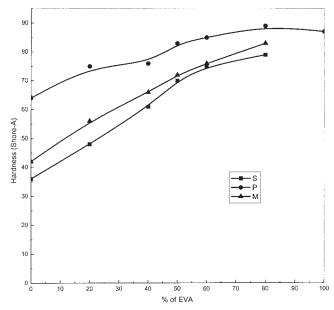
**Figure 12** Effect of the blend ratio and different crosslinking systems on the hardness of the SBR/EVA blends.
