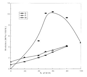
Figure 9 Effect of the blend ratio and different crosslinking systems on the modulus of the SBR/EVA blends.
