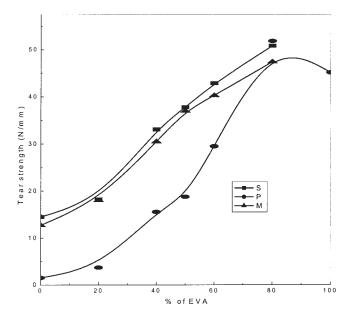
**Figure 11** Effect of the blend ratio and different crosslinking systems on the tear strength of the SBR/EVA blends.
